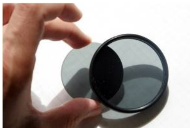
Light through two polarizers
